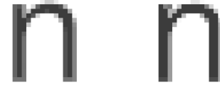
Figure 11. Helvetica 'n' rendered from an ADF without (left) and with (right) automatic hinting of left and bottom edges by darkening pixels where the gradient of the distance field indicates a left or bottom edge and lightening pixels corresponding to right and top edges to maintain stroke weight.
