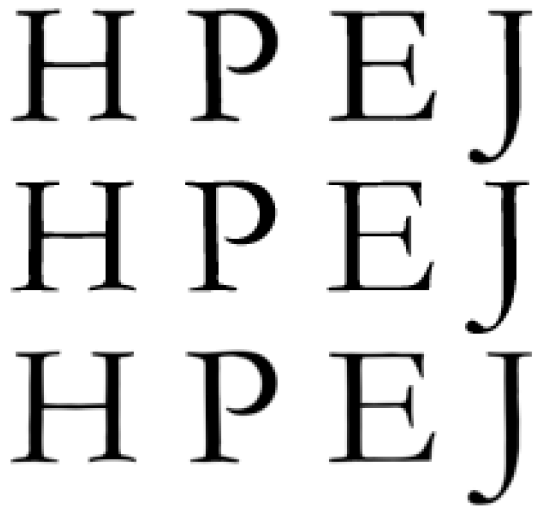
Figure 6. Garamond glyphs at display type sizes rendered, from top to bottom, by 16x supersampling with a Gaussian filter, Adobe Illustrator with hinting and supersampling, and the unhinted single sample per pixel ADF method of Section 4.2.2. These images were digitally captured from the display device and then pixel replicated 3x. Note the ragged left edges of the vertical stems of the H, P, and J, the ragged horizontal bar of the H, and the ragged top bars of the P and E for the supersampled and Adobe Illustrator renderings. The ADF method produces smoother edges while maintaining good contrast.
