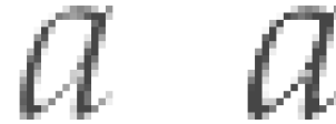
Figure 12. Palatino 'a' rendered from an ADF without (left) and with (right) automatic hinting to thicken thin strokes by slightly darkening pixels where the gradient of the distance field changes abruptly between adjacent pixels.
