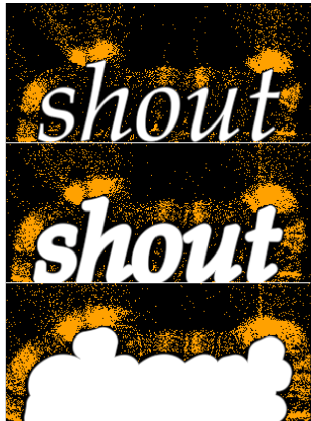
Figure 14. Three frames from an animated vignette which uses the ADF to attract and repel particles in a real time particle system and uses the implicit nature of the distance field to create offset surfaces from the glyphs. The distance field permits complex topological changes that would be difficult to model with outline-based fonts.
