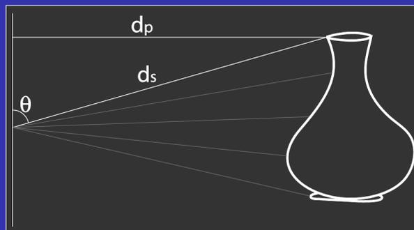
Use scanner geometry to derive perpendicular distances from line-of-sight distances
